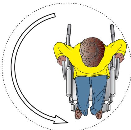
Figure 1. A turning circle for wheelchairs<sup>5</sup>
