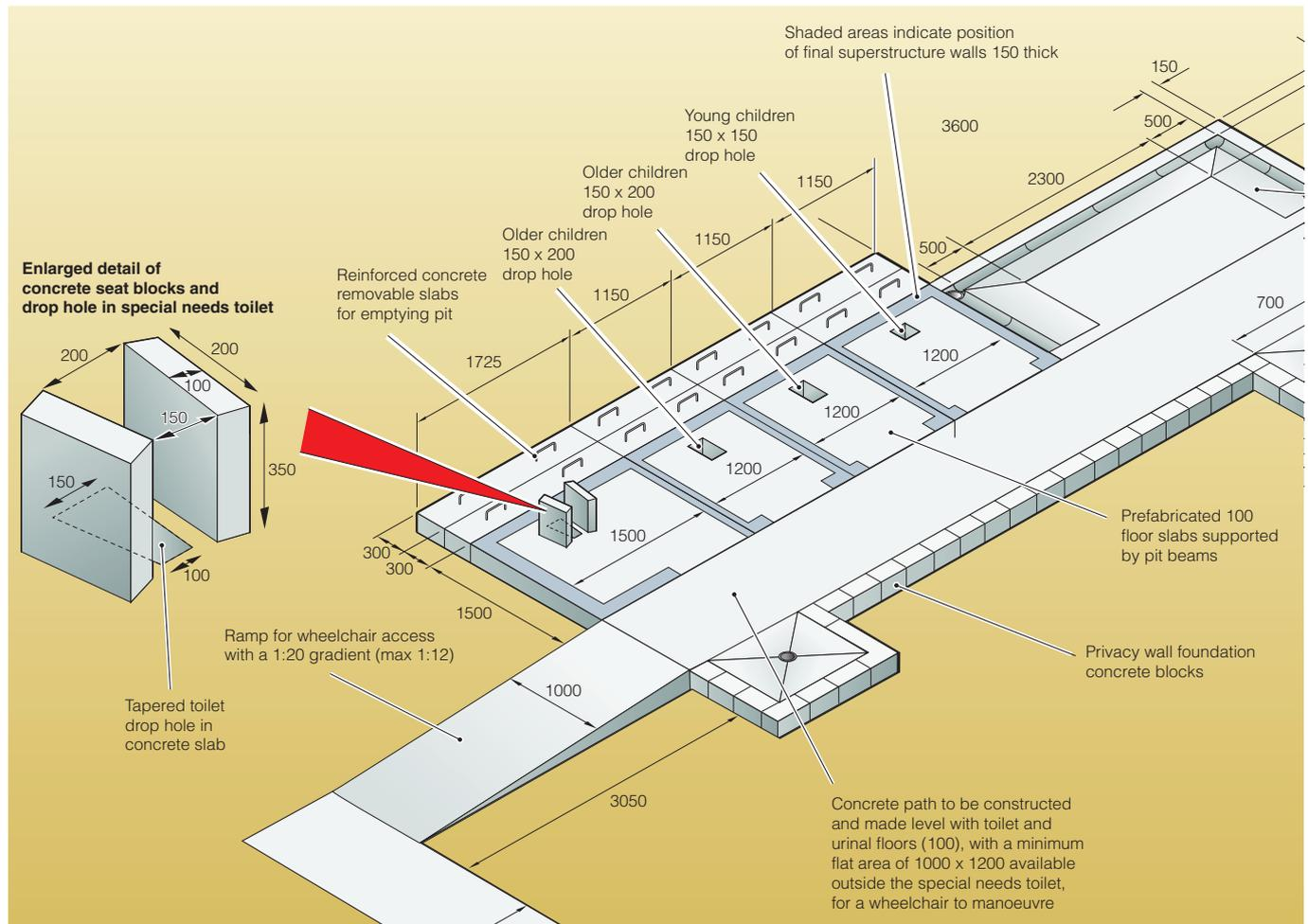
Figure 2. Floor construction: cement block or burnt brick with concrete slab (boys)<sup>9</sup>
