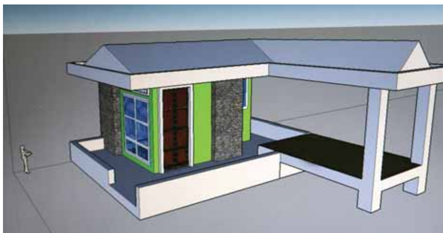
Computer sketch for the new library with the beruqaq on the right. Note the high contrast colours to help students with low-vision.
